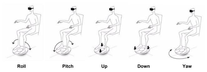
Below is the 3D axis définition used by the 3dRudder to move or rotate in the 3D world :
