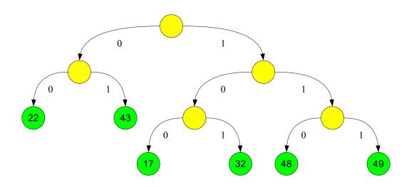
Figure 2.4: Huffman tree for the data stream in figure 2.2.
